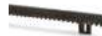
ROA6 M4 25x20x1000 mm SLOTTED NYLON RACK WITH METAL INSERT FOR GATES WEIGHING UP TO 500 kg. PC/PACK 10
